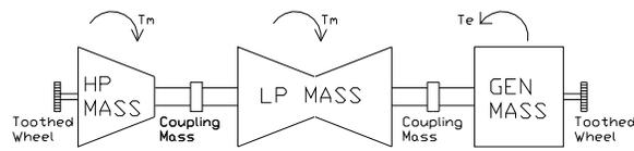
Fig 4-4: Turbine-Generator Spring-Mass Model
